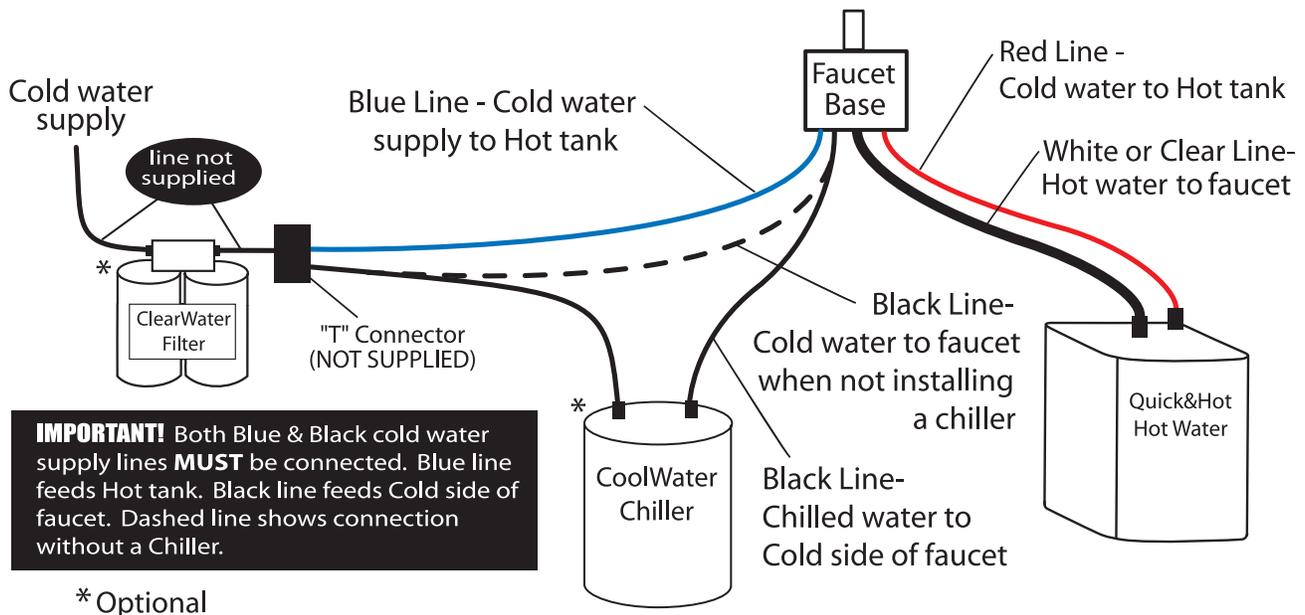
**IMPORTANT!** Both Blue & Black cold water supply lines **MUST** be connected. Blue line feeds Hot tank. Black line feeds Cold side of faucet. Dashed line shows connection without a Chiller.
