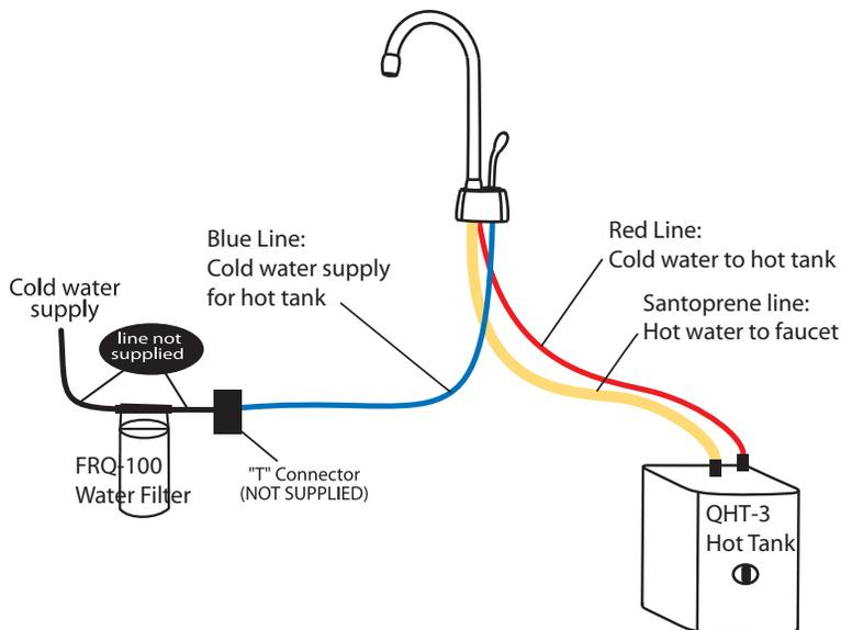
**NOTE:** Copper lines are color coded with red or blue tape and are referred to as Red line and Blue line.
