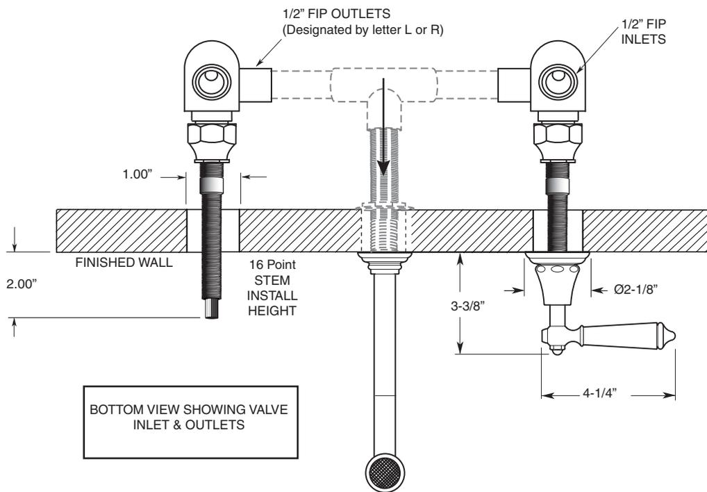
BOTTOM VIEW SHOWING VALVE INLET & OUTLETS
