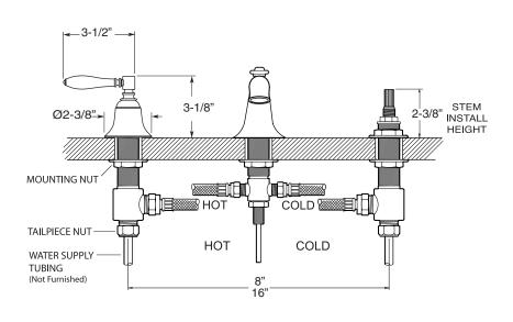
NOTE: Spout and valves install through 1-1/4" diameter holes
