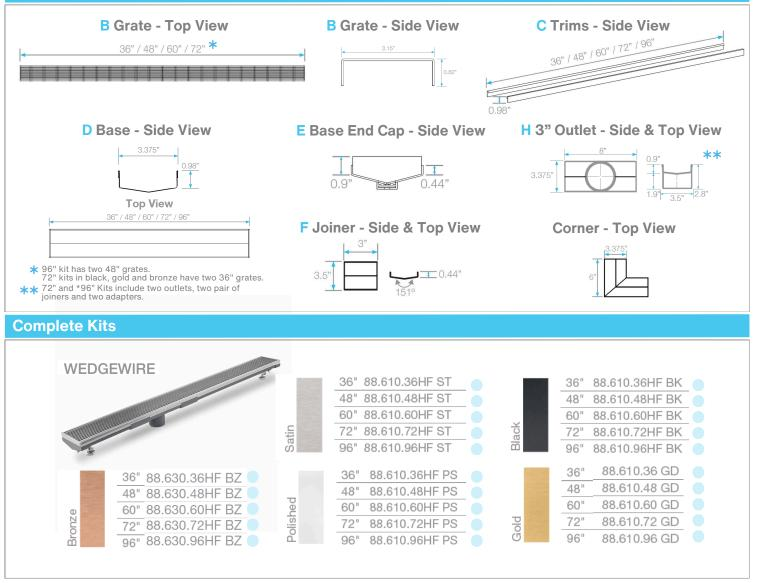
Note: Installer must verify all rough-in dimensions prior to installation and consult local and national codes. Conformity and compliance to local and national codes are the responsibility of the installer. Dimensions are subject to manufacturers tolerance and change without notice. We can assume no responsibility for use of superseded or voided data. Contact us If you have any question at: techsupport@qm-us.com
