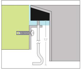
DESCRIPTION Flush-mount Installation Kit TECHNICAL INFORMATION 16 GA. 304 Stainless Steel Angle Stainless Steel 12" Height Adjusting Screw Stainless Steel Lock Washers Aluminum Anchors • INCLUDED PARTS #8-32 Screw 12" Height Adjusting Screw #8 Lock Washer #8-32 Standoff #8-32 #8 #8-32
