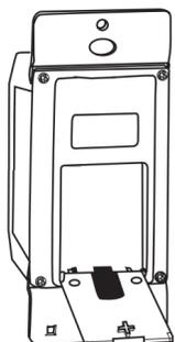
Programming controls hidden discretely behind door on front panel.
