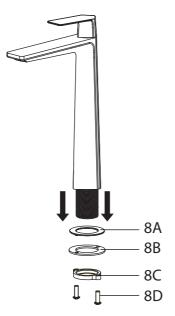
Remove the mounting screws (8D), mounting nut (8C), metal washer (8B), and rubber washer (8A) from the mounting pipe
