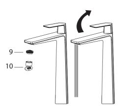
After installing faucet, remove aerator (9) with included aerator key (10). Turn water on for 30 seconds to remove any debris. Reassemble aerator (9)
