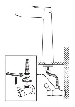
Connect flex water supply lines to angle stops and tighten with adjustable wrench. Turn on both hot and cold main valve
