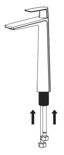
Place faucet on a soft cloth, spout facing up. Attach the waterlines into the base of the faucet (HAND-TIGHTEN ONLY) (A)Hot side left (B)Cold side right
