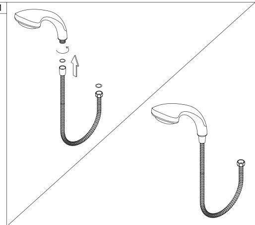
1. Connect tapered end of hose to hand shower seat the washer, if provided, firmly into the hose nut. from the end of the hose that screws onto the hand shower. Carefully align the thread of the tapered end of the hose directly to the hand shower. Hand tighten - do not use a wrench or pliers. Then place the hand shower into the shower arm mount. Rotate the shower arm mount into desired position to hold the hand shower.
