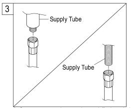
3. Connect sprayer hose to the partially threaded inlet stem on the supply tube.
