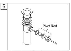
6. Place pivot rod into pivot rod opening. Slide pivot nut over pivot rod and thread it on the drain body. Tighten firmly.
