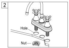
Set the faucet in place, insert the inlet shanks through the sink holes, and press down.Assemble the washers and locknuts on the inlet shanks, and then tighten the nuts with hand.
