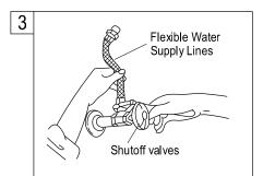
Connect the water supply lines. Before connecting the supply lines, apply pipe joint compound to the threads on the inlet shanks and shut off valves with an adjustable wrench.
