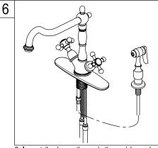
6. Insert the hose through the guide and attach to the fitting on the bottom of the faucet. Attach spray head to the hose.
