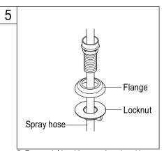
5. For model is with spray head and hose. Place the spray guide through the fourth hold in the sink, screw the locknut onto the shank and tighten firmly.
