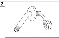
2. Wrap threads on one end of shower rod male nipple with 4 to 6 wraps of Teflon's tape.
