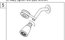
5. Wrap Teflon's tape around all the threads on shower rod and hand tighten the shower head clockwise.
