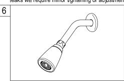
6. Turn the water on and check for leaks, any leaks will require minor tightening or adjustment. If the shower head leaks at the connection to the thread shower arm, tighten the connection some more by using a wrench.
