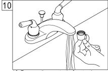
10. Remove the aerator before turning on your new faucet for the first time. This is to prevent any deposits from clogging your aerator. Allow both hot and cold water to run for one minute. Replace aerator.
