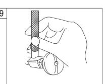
9. Turn on water supply valves and check for leaks, especially at hook-ups to supply
