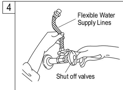
4. Connect the water supply lines. Before connecting the supply lines, apply pipe joint compound to the threads on the inlet shanks and shut off valves with an adjustable wrench.
