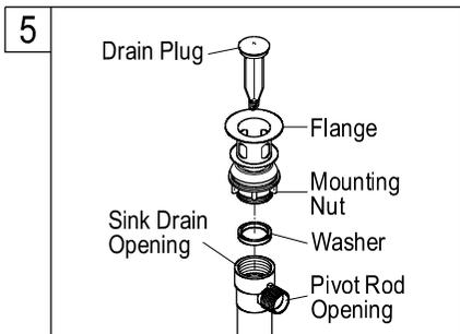
5. Install flange body up through the drain opening, hold the drain flange body in position with pivot rod opening facing the back of sink and hand tighten the mounting nut.
