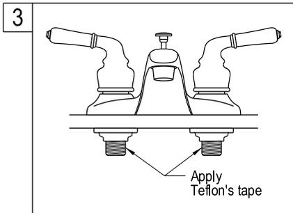
3. Apply Teflon's tape to inlet shanks and connect supply lines.
