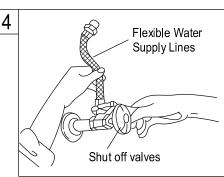
Connect the water supply lines. Before connecting the supply lines, apply pipe joint compound to the threads on the nlet shanks and shut off valves.
