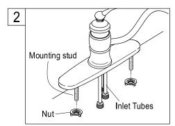
Set the faucet in place, insert the inlet mounting stud through the sink holes, and press down. Assemble the nuts on the inlet mounting stud, and then tighten the nuts by hand.
