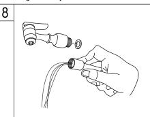
8.Remove spray head by unscrew the sprayer counter-clockwise. To flush debris to avoid clogs in plumbing line by allow both hot and cold water running to flush for at least one minute. This process will help to prevent any clogs and deposits from clogging the diverter, or into hose and spray head. Reinstall spray head when done, press on sprayer trigger to release any air pressure inside the waterway.
