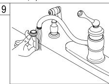
9. Remove the aerator before turning on your new faucet for the first time, let hot and cold water run for at least 1 minute, replace aerator this will prevent debris in the line from cogging the aerator.
