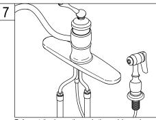
7. Insert the hose through the guide and attach to the fitting on the bottom of the faucet. Attach spray head to the hose.
