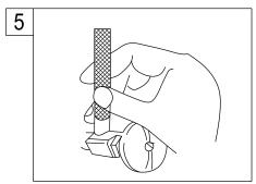
5. Turn on water supply valves and check for leaks, especially at hook-ups to supply lines.
