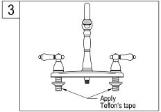
3. Apply Teflon's tape to inlet shanks and connect supply lines.
