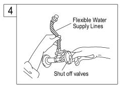
4. Connect the water supply lines. Before connecting the supply lines, apply pipe joint compound to the threads on the inlet shanks and shut off valves.
