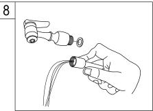
8.Remove spray head by unscrew the sprayer counter-clockwise. To flush debris to avoid clogs in plumbing line by allow both hot and cold water running to flush for at least one minute. This process will help to prevent any clogs and deposits from clogging the diverter, or into hose and spray head. Reinstall spray head when done, press on sprayer trigger to release any air pressure inside the waterway.
