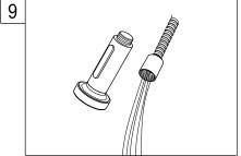
9. Pull the spray hose through the spout and secure the end into the drain, or have a secure party hold the spray hose, and turn on the faucet and flush for one minute.
