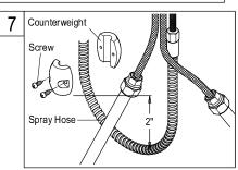
7. Install counterweight set on the spray hose. Adjust the counterweight at least 2" higher then the bottom line as illustrated. Fix with screws tightly.
