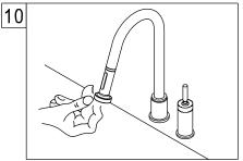
10. Attach spray head to the large end of the stainless steel hose. Insert spray head onto faucet body.
