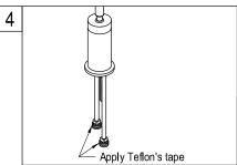
4. Apply Teflon's tape to inlet shanks and connect supply lines.
