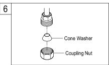
6. if you have 3/8" supply tubes, use the 3/8" friction ring that is in the parts bag. If you have 1/2" supply tubes, use the 1/2" friction ring that is in the parts bag. Place the friction ring and cone washer into the coupling nut as shown in the above illustration, and then connect. HAND TIGHTEN ONLY, AND BE CAREFUL NOT TO OVER TIGHTEN.
