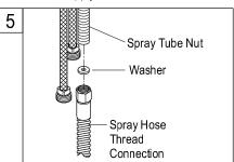
5. Wrap Teflon's tape on the spray hose thread connection and connect the spray hose to spray tape and secure with spray tube nut. Tighten with wrench carefully.
