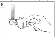
8. Turn on hot and cold water at the valves and check for leaks. If leak is found, slightly tighten connection. Do not overtighten.
