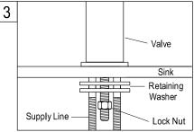
3. Install Valve. Insert valve through sink. Position valve so that the longer supply line is on the left side. Place retainer washer over the threaded stem and thread nut into place. Tighten nut using enclosed wrench. Be sure to keep rubber washer above the sink surface.
