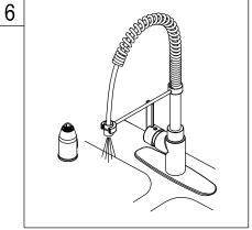
6. Important: After installation is complated. Turn on water supply and allow both hot and cold water to run for at least one minute each. While water is running, check for leaks.
