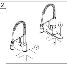
2. Place assembly(1) or flange(2) on bottom of new faucet (Optional). Position faucet through mounting hole.
