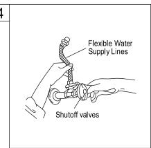
4. Connect the water supply lines. Before connecting the supply lines, apply pipe joint compound to the threads on the inlet shanks and shut off valves with an adjustable wrench.
