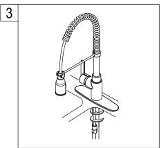
3. Secure the faucet to sink by installing rubber washer, steel washer and nut into it. Tighten with wrench.
