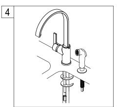
4. Secure the faucet to sink by installing rubber washer, steel washer and nut into it. Tighten with wrench.
