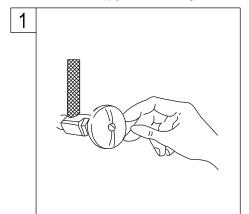
1. Shut off hot and cold water supply under sink. Plug sink drain with doth to avoid losing small parts. Remove old faucet.
