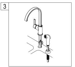
3. For Models with a spray support. Mount spray support on far right hole of the sink. Insert spray hose down through the support and up through the center hole of sink. Attach spray hose to spray hose nipple.
