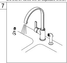
7. Important: After installation is complated. Turn on water supply and allow both hot and cold water to run for at least one minute each. While water is running, check for leaks.
