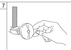
7. Turn on hot and cold water at the valves and check for leaks. If leak is found, slightly tighten connection. Do not overtighten.
