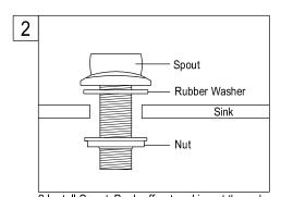
2.Install Spout. Back off nut and insert through sink. Be sure to keep rubber washer above the sink surface. From underneath sink, attach nut to spout and tighten by hand. Be careful not to overtighten.
