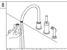
8. Remove the aerator before turning on your new faucet for the first time. This is to prevent any deposits from clogging your aerator. Allow both hot and cold water to run for one minute. Replace aerator.
