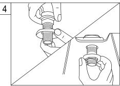
4.Install Sprayer: Insert hose guide through guide flange and snap into place. Install guide through sink and attach with mounting nut.
