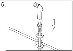
5. Attached sprayer head, to hose, and hand tighten only. Plumbers tape is not required. Drop sprayer hose through hose guide and let it rest in place.
