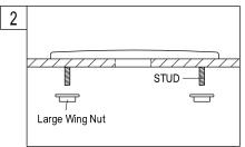
2.For Installation using the deck plate, Thread mounting bolts stud into deck plate, place plastic plate under the deck plate smooth side down and place the plates on deck. Making sure to align center hole on plate with center hole on counter or sink, as to allow for easy insertion of spout
