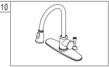
10. Insert the spray head onto the faucet body to assure the hose assembled correctly.
