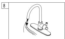
8.Pull the stainless steel hose assembly out of the spout and hold into the sink, turn faucet on to the full mixed position, let the water run for at least one minutes to flush the lines.
