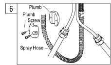
6.Under the sink, attach the plumb onto the spray hose. Adjust the plumb at least 2" higher than the bottom lines and fix with screws tightly.
