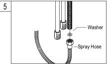
5.Pull the stainless steel hose up through the faucet till the attachment nut is up against the bottom of the faucet shank, from underneath slip on rubber gasket and brass washer onto the shank then thread with brass nut, tighten lightly with hand and check faucet alignment, then retighten with wrench.
