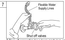
7. Once all connection have been made turn on watersupply and check for leaks.
