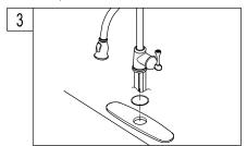
3.Insert o-ring into bottom groove of faucet, from above insert faucet, making sure to center the front of the faucet.
