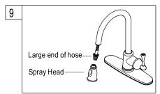
9. Attach the spray head to the large end of the stainless steel hose and press the soft oval button to assure the Spray head is working.
