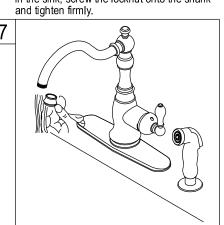
7.Remove the aerator before turning on your new faucet for the first time. This is to prevent any deposits from clogging your aerator. Allow both hot and cold water to run for one minute. Replace aerator.
