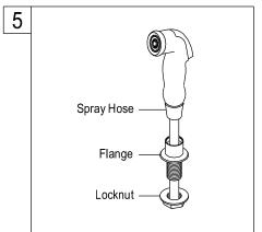
5. For model with spray head and hose. Place the spray guide through the fourth hole in the sink, screw the locknut onto the shank
