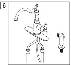
6. For model with spray head and hose. Place the spray guide through the fourth hole in the sink, screw the locknut onto the shank and tighten firmly.
