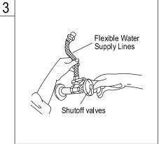
3. Connect the water supply lines. Before connecting the supply lines, apply pipe joint compound to the threads on the inlet shanks and shut off valves with an adjustable wrench.
