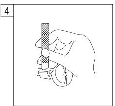
4. Turn on water supply valves and check for leaks, especially at hook-ups to supply lines.
