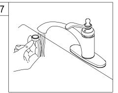
7. Remove the aerator before turning on your new faucet for the first time. This is to prevent any deposits from clogging your aerator. Allow both hot and cold water to run for one minute. Replace aerator.
