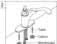
through the sink holes, and press down. Assemble the washers and locknuts on the inlet studs, and then tighten the nuts with hand.
