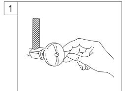
1.Turn off both sides "Hot" and "Cold" at water supply shut off valves under the sink. Plug drain hole of the sink with a piece of cloth to avoid small parts from dropping into drain during installation.
