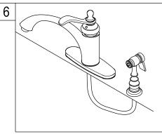
6. Insert the hose through the guide and attach to the fitting on the bottom of the faucet. Attach spray head to the hose.
