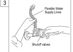
3. Connect the water supply lines. Before connecting the supply lines, apply pipe joint compound to the threads on the inlet shanks and shut off valves.
