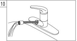
10. Pull the spray hose through the spout and secure the end into the drain, or have a secure party hold the spray hose, and turn on the faucet and flush for one minute.
