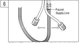
6. Note: if faucet supply lines need to be bent, grip tube at point of bend with right hand, firmly and slowly pull tube into position using rounded bend with left hand. Extreme care must be exercised. Follow instructions exactly. Kinked tubes will void warranty.
