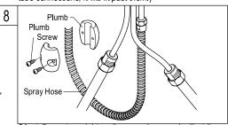
8.Install counterweight on the spray hose and adjust the counterweight at least 2"higher than the bottom line as illustrated. Fix with screws tightly.
