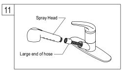
11. Attach spray head to the large end of the stainless steel hose. Insert spray head onto faucet body.
