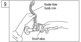
9. After completed the installation, be sure the faucet is in off position before turning on the hot and cold supply valves to check for leaks, especially at hook ups to supply lines. Tightening nits slightly will stop any minor leaks.
