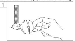
1. Turn off water supply valves under the sink. Cover the sink drain so that no small parts are lost down it. Remove your old faucet. Caution: Do not damage your old water supply lines. Clean the surface of the sink in preparation for installing the new faucet.
