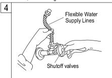
4. Connect the water supply lines. Before connecting the supply lines, apply pipe joint compound to the threads on the inlet shanks and shut off valves with an adjustable wrench.
