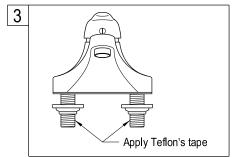
3. Apply Teflon's tape to inlet shanks and connect supply lines.
