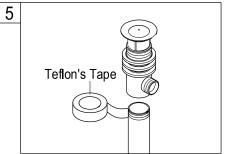
5. Thread mounting nut and bottom gasket onto drain body. Wrap top threaded end of the drain body with plumbers' tape.
