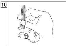
10. Turn on water supply valves and check for leaks, especially at hook-ups to supply lines.
