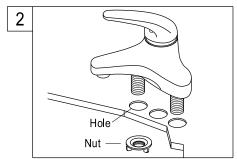
2. Set the faucet insert the inlet studs through the sink plate holes, and press down. Assemble the washers and locknuts on the inlet shanks, and then tighten the nuts with hand.
