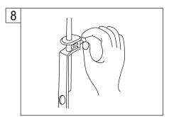
8. With lift rod in position on the faucet, insert lift rod through lift rod strap and secure with the clevis screw.
