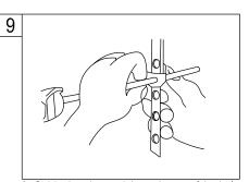
9. Guide the pivot rod through one of the holes on the lift rod strap and secure it with the spring clip. Then adjust the height of the lift rod by resetting the clevis screw.
