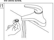
11. Remove the aerator before turning on your new faucet for the first time. This is to prevent any deposits from clogging your aerator. Allow both hot and cold water to run for one minute. Replace aerator.
