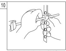
10. Guide the pivot rod through one of the holes on the lift rod strap and secure it with the spring dip. Then adjust the height of the lift rod by resetting the devis screw.
