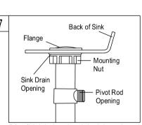
7. Install drain body up through the drain opening and reattach the flange onto drain body, holding the drain body in position with pivot rod opening facing the back of sink. Tighten the mounting nut by hand.
