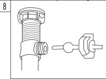
Place pivot rod into pivot rod opening. Slide pivot nut over pivot rod and thread it on the drain body. Tighten firmly.
