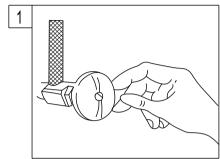
Shut off hot and cold water supply under sink.
