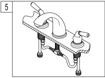
Connect the flexible tubes from the supply shank side port to the Spout Tee. Also reattach the supply lines, turn on the water supply, and check for leaks.
