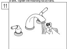
Remove the aerator before turning on your new faucet for the first time. Allow both hot and cold water to run for one minute. Replace aerator.
