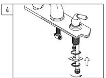
4. Hold the handles in proper position. Make sure that the top of the faucet handles is 5/8" above the top of the sink. Mount the metal washer and locknut from underneath the sink. Than reposition escutcheons as necessary to a desired height.
