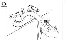
10. Remove the aerator before turning on your new faucet for the first time. This is to prevent any deposits from clogging your aerator. Allow both hot and cold water to run for one minute. Replace aerator.
