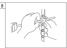
8. Guide the pivot rod through one of the holes on the lift rod strap and secure it with the spring clip. Then adjust the height of the lift rod by resetting the clevis screw.
