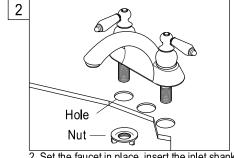
2. Set the faucet in place, insert the inlet shanks through the sink holes, and press down. Assemble the washers and locknuts on the inlet shanks, and then tighten the nuts with hand.
