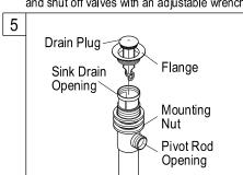
5. Install drain body up through the drain opening and reattach the flange onto drain body, holding the drain body in position with pivot rod opening facing the back of sink. Tighten the mounting nut by hand.
