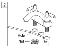
2. Set the faucet in place, insert the inlet shanks through the sink holes, and press down.
