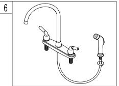
6. Insert the hose through the guide and attach to the fitting on the bottom of the faucet. Attach spray head to the hose.
