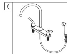
5. For model is with spray head and hose. Place the spray guide through the fourth hold in the sink, screw the locknut onto the shank and tighten firmly.
