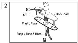
Place deck plate in proper position, put hose and supply tubes through center hole of deck plate. Install hold down studs onto brass deck plate by sliding stud into the notched receptacle on the base plate. Place plastic plate under the deck plate smooth side down.
