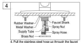
until the attachment nut is up against the bottom of the faucet shank. Install rubber washer and metal washer on the faucet shank and secure with brass nut, tighten wrench tight. (Have patience when slipping the brass nut past the water tube connections, it will fit past them.)
