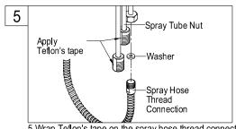
5. Wrap Teflon's tape on the spray hose thread connection and connect the spray hose to spray tape and secure with spray tube nut. Tighten with wrench carefully.
