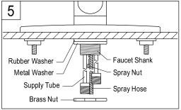
5. Pull the stainless steel hose up through the faucet till the attachment nut is up against the bottom of the faucet shank, From underneath slip on Rubber gasket and brass washer onto the shank then thread with Brass nut, tighten lightly with hand and check faucet alignment, then retighten with wrench.
