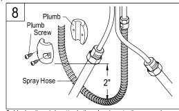
8. Under the sink, attach the plumb onto the spray hose. Adjust the plumb at least 2" higher than the bottom lines and fix with screws tightly.
