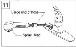
11. Attach the spray head to the large end of the stainless steel hose and press the soft oval button to assure the shower head is working.
