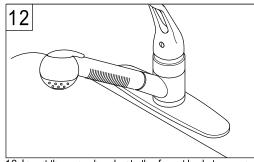
12. Insert the spray head onto the faucet body to assure the hose assembled correctly.
