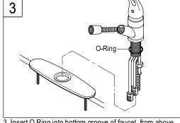
3. Insert O Ring into bottom groove of faucet, from above insert faucet, making sure to center the front of the faucet. (please note, your Kingston brass faucet has a swivel range of 105°, so it is important that you take the time to align the faucet properly, by making sure that the handle faces forward at center closed position and that spout swivel range is centered.)
