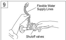
9. Once all connection have been made turn on water supply and check for leaks.
