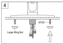
4. Secure faucet by threading wing nut onto mounting bolts and tighten until deck plate feels firmly secure.
