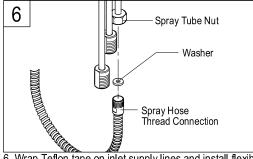
6. Wrap Teflon tape on inlet supply lines and install flexible water supply lines (not included), and secure with spray tube nut, tighten with wrench carefully.
