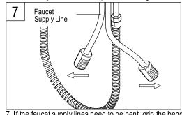
7. If the faucet supply lines need to be bent, grip the bend point of tube with right hand, slowly and firmly pull the tube into position using rounded bend with left hand. Extremely care must be exercised; kinked tubes will void the warranty
