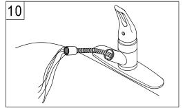
10. Pull the stainless steel hose assembly out of the spout and hold into the sink, turn faucet on to the full mixed position. let the water run for at least 1 minutes to flush the lines.
