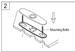
2. For Installation using the Deck plate, Thread mounting bolts(62) into deck plate, place plastic plate under the deck plate smooth side down and place the plates on deck. Making sure to align center hole on plate with center hole on counter or sink, as to allow for easy insertion of spout.
