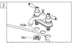
2. Set the faucet in place, insert the inlet shanks through the sink holes, and press down.
