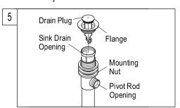
5. Install drain body up through the drain opening and reattach the flange onto drain body, holding the drain body in position with pivot rod opening facing the back of sink. Tighten the mounting nut by hand.
