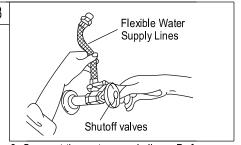
3. Connect the water supply lines. Before connecting the supply lines, apply pipe joint compound to the threads on the inlet shanks and shut off valves with an adjustable wrench.
