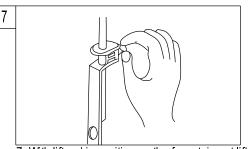
7. With lift rod in position on the faucet, insert lift rod through lift rod strap and secure with the clevis screw.
