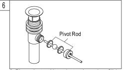
6. Place pivot rod into pivot rod opening. Slide pivot nut over pivot rod and thread it on the drain body. Tighten firmly.
