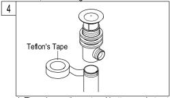
4. Thread mounting nut and bottom gasket onto drain body. Wrap top threaded end of the drain body with teflon's Tape.
