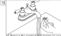
10. Remove the aerator betore turning on your new faucet for the first time. This is to prevent any deposits from clogging your aerator. Allow both hot and cold water to run for one minute. Replace aerator.
