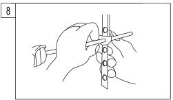
8. Guide the pivot rod through one of the holes on the lift rod strap and secure it with the spring clip. Then adjust the height of the lift rod by resetting the clevis screw.
