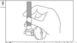
9. Turn on water supply valves and check for leaks, especially at hook-ups to supply lines.
