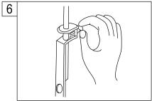
6. With lift rod in position on the faucet, insert lift rod through lift rod strap and secure with the clevis screw.
