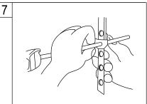
7. Guide the pivot rod through one of the holes on the lift rod strap and secure it with the spring clip. Then adjust the height of the lift rod by resetting the clevis screw.
