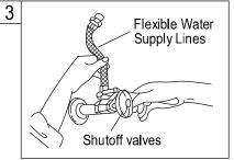
3. Connect the water supply lines. Before connecting the supply lines, apply pipe joint compound to the threads on the inlet shanks and shut off valves with an adjustable wrench.
