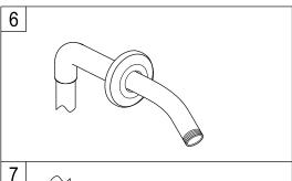
6.Place the shower flange over shower arm. Apply pipe compound to the threads on the long end of the shower arm. Screw that end into the shower riser elbow. Push flange against the wall.
