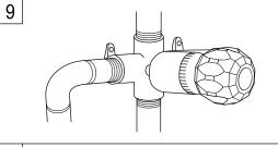
9. Turn on water supply and check connections for leaks. Place handle on valve stem and flush lines by running hot and cold water uninterrupted for one minute.
