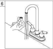
6. Remove the aerator before turning on your new faucet for the first time. This is to prevent any deposits from clogging your aerator. Allow both hot and cold water to run for one minute. Replace aerator.
