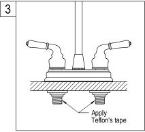
3. Apply Teflon's tape to inlet shanks and connect supply lines.
