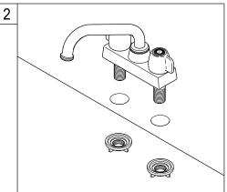
2. Set the faucet in place, insert the inlet shanks through the sink holes, and press down. Assemble the washers and locknuts on the inlet shanks, and then tighten the inuts with hand.
