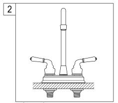
2. Set the faucet in place, insert the inlet shanks through the sink holes, and press down. Assemble the washers and locknuts on the inlet shanks, and then tighten the nuts with hand.
