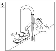
5. Remove the aerator before turning on your new faucet for the first time. This is to prevent any deposits from clogging your aerator. Allow both hot and cold water to run for one minute. Replace aerator.
