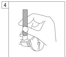
4. Turn on water supply valves and check for leaks, especially at hook-ups to supply lines.
