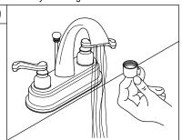
9. Remove the aerator before turning on your new faucet for the first time. This is to prevent any deposits from clogging your aerator. Allow both hot and cold water to run for one minute. Replace aerator.
