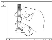
8. Turn on water supply valves and check for leaks, especially at hook-ups to supply lines.
