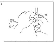
7. Guide the pivot rod through one of the holes on the lift rod strap and secure it with the spring dip. Then adjust the height of the lift rod by resetting the clevis screw.
