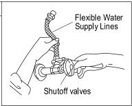
3. Connect the water supply lines. Before connecting the supply lines, apply pipe joint compound to the threads on the inlet shanks and shut off valves with an adjustable wrench.
