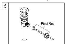
5. Place pivot rod into pivot rod opening. Slide pivot nut over pivot rod and thread it on the drain body. Tighten firmly.
