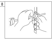
8. Guide the pivot rod through one of the holes on the lift rod strap and secure it with the spring clip. Then adjust the height of the lift rod by resetting the clevis screw.
