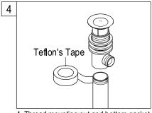
4. Thread mounting nut and bottom gasket onto drain body. Wrap top threaded end of the drain body with plumbers' tape.
