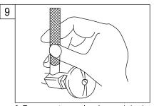
9. Turn on water supply valves and check for leaks, especially at hook-ups to supply lines.
