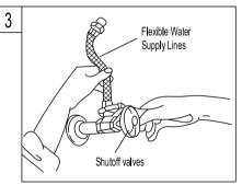
3. Connect the water supply lines. Before connecting the supply lines, apply pipe joint compound to the threads on the inlet shanks and shut off valves.
