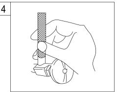
4. Turn on water supply valves and check for leaks, especially at hook-ups to supply lines.
