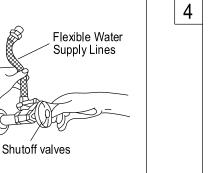
3. Connect the water supply lines. Before connecting the supply lines, apply pipe joint compound to the threads on the inlet shanks and shut off valves.
