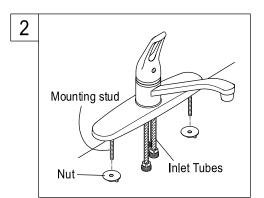
2. Set the faucet in place, insert the inlet shanks through the sink holes, and press down. Assemble the mounting stud and nuts on the inlet shanks, and then tighten the nuts with hand.
