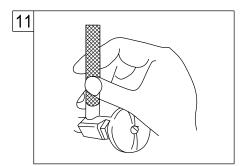
11. Turn on water supply valves and check for leaks, especially at hook-ups to supply lines.
