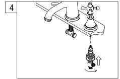
4. Hold the handles in proper position. Make sure that the top of the faucet handles is 5/8" above the top of the sink. Mount the metal washer and locknut from underneath the sink. Then reposition escutcheons as necessary to a desired height.
