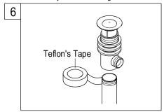
6. Thread mounting nut and bottom gasket onto drain body. Wrap top threaded end of the drain body with teflon's tape.
