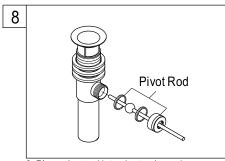
8. Place pivot rod into pivot rod opening.
