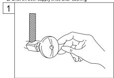
Shut off hot and cold water supply under sink.
