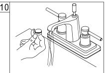
10. Remove the aerator before turning on your new faucet for the first time. This is to prevent any deposits from clogging your aerator. Allow both hot and cold water to run for one minute. Replace aerator.
