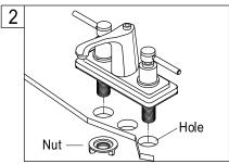
2. Set the faucet in place, insert the inlet shanks through the sink holes, and press down. Assemble the washers and locknuts on the inlet shanks, and then tighten the nuts with hand.
