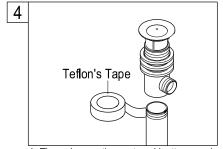
4. Thread mounting nut and bottom gasket onto drain body. Wrap top threaded end of the drain body with plumbers' tape.
