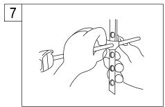
7. Guide the pivot rod through one of the holes on the lift rod strap and secure it with the spring dip. Then adjust the height of the lift rod by resetting the clevis screw.
