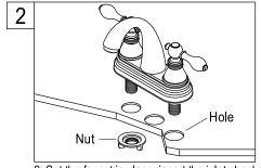
2. Set the faucet in place, insert the inlet shanks through the sink holes, and press down. Assemble the washers and locknuts onto the inlet shanks, and then tighten the nuts with hand.
