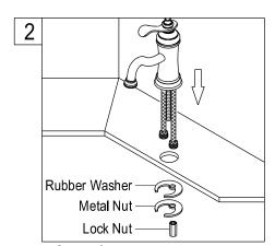
2. Set the faucet insert the inlet shanks through the sink plate holes, and press down. Assemble the washers and locknuts on the inlet shanks, and then tighten the nuts with hand.
