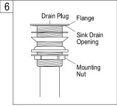
6. Install drain body up through the drain opening and reattach the flange onto drain body, holding the drain body in position with pivot rod opening facing the back of sink. Tighten the mounting nut by hand.
