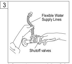
Connect the water supply lines. Before connecting the supply lines, apply pipe joint compound to the threads on the inlet shanks and shut off valves.
