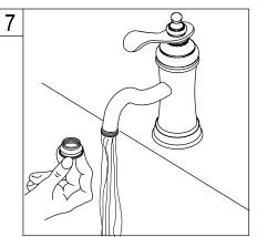
7. Remove the aerator before turning on your new faucet for the first time. This is to prevent any deposits from clogging your aerator. Allow both hot and cold water to run for one minute. Replace aerator.
