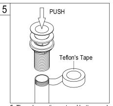
5. Thread mounting nut and bottom gasket ontodrain body. Wrap top threaded end of the drain body with plumbers' tape.
