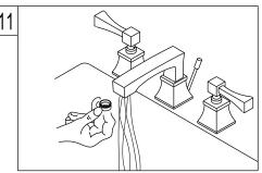
11. Remove the aerator before turning on your new faucet for the first time. This is to prevent any deposits from clogging your aerator. Allow both hot and cold water to run for one minute. Replace aerator.
