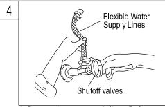
4. Connect the water supply lines. Before connecting the supply lines, apply pipe joint compound to the threads on the inlet shanks and shut off valves with an adjustable wrench.
