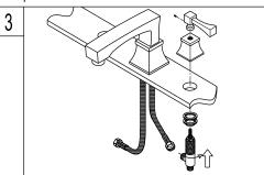
3. Hold the handles in proper position. Make sure that the top of the faucet handles is 5/8" above the top of the sink. Mount the metal washer and locknut from underneath the sink. Than reposition escutcheons as necessary to a desired height.
