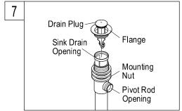
7. Install drain body up through the drain opening and reattach the flange onto drain body, holding the drain body in position with pivot rod opening facing the back of sink. Tighten the mounting nut by hand.
