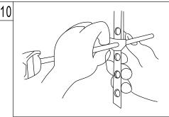
10. Guide the pivot rod through one of the holes on the lift rod strap and secure it with the spring clip. Then adjust the height of the lift rod by resetting the clevis screw.
