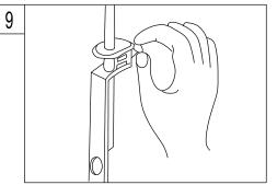
9. With lift rod in position on the faucet, insert lift rod through lift rod strap and secure with the clevis screw.
