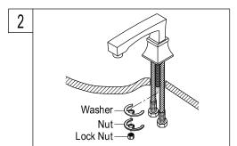
Install new faucet spout through the center hole of sink. Place mounting washer on spout shank and attach with spout shank locknut.
