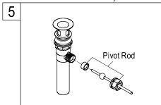
5. Place pivot rod into pivot rod opening. Slide pivot nut over pivot rod and thread it on the drain body. Tighten firmly.
