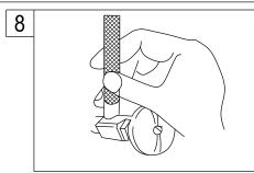
8. Turn on water supply valves and check for leaks, especially at hook-ups to supply lines.
