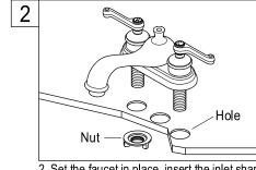
2. Set the faucet in place, insert the inlet shanks through the sink holes, and press down. Assemble the washers and locknuts onto the inlet shanks, and then tighten the nuts with hand.
