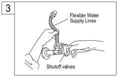
3. Connect the water supply lines. Before connecting the supply lines, apply pipe joint compound to the threads on the inlet shanks and shut off valves with an adjustable wrench.
