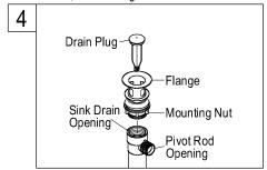
4. Install flange body up through the drain opening, hold the drain flange body in position with pivot rod opening facing the back of sink and hand tighten the mounting nut.
