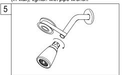
5. Wrap teflon's tape around all the threads on shower rod and hand tighten the showerhead clockwise.
