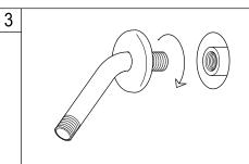
3. Thread the male nipple into female nipple (in wall), tighten with pipe wrench.
