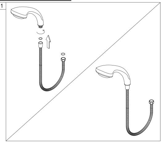
Put a washer to the cone shape hose nut and hand tightens the hand shower clockwise.
