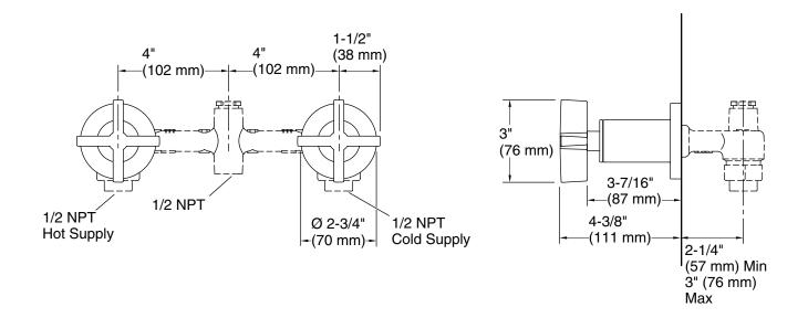
Technical Information All product dimensions are nominal. Notes Install this product according to the installation instructions. ADA, OBC, CSA B651 compliant when installed to the specific requirements of these regulations.
